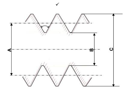
A = Pitch diameter / Effective diameter  $\checkmark$
