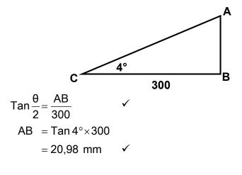
$$d = D - 2(AB) \qquad \checkmark = 200 - 2(20,98) \qquad \checkmark = 158,04 \text{ mm} \qquad \checkmark$$
