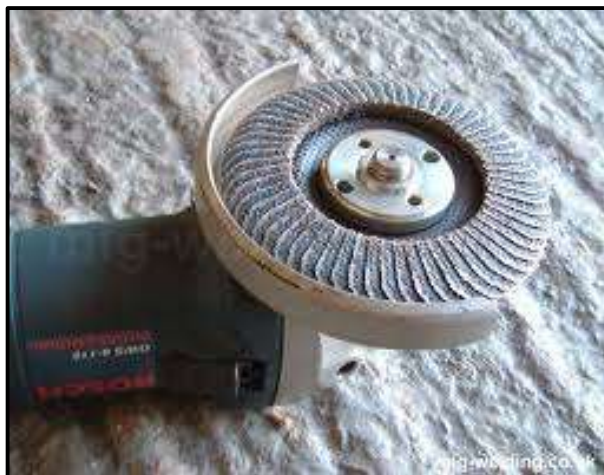
Figure 8: Flapper disc mounted on angle grinder
