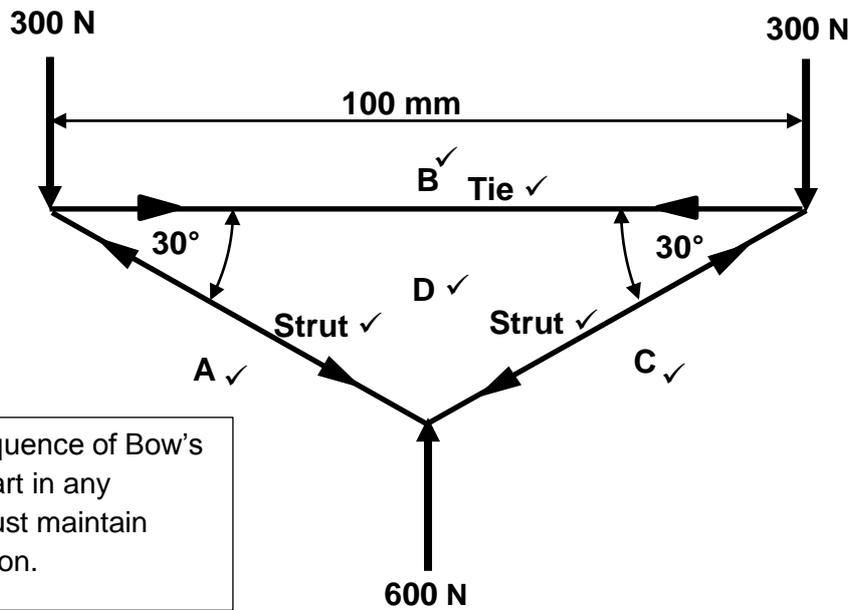
**NOTE:** The sequence of Bow's notation can start in any position, but must maintain clockwise rotation.
