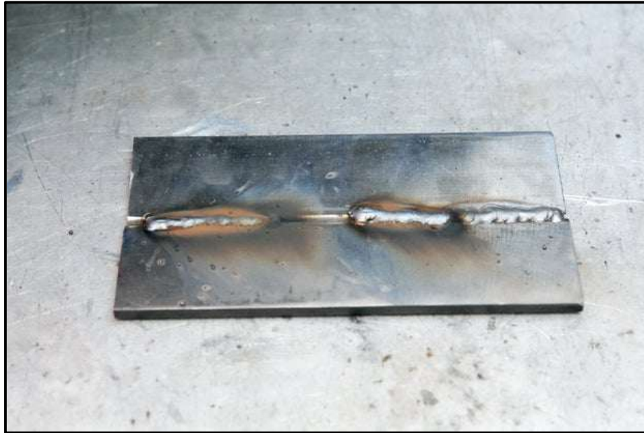
Figure 16: Start weld runs
