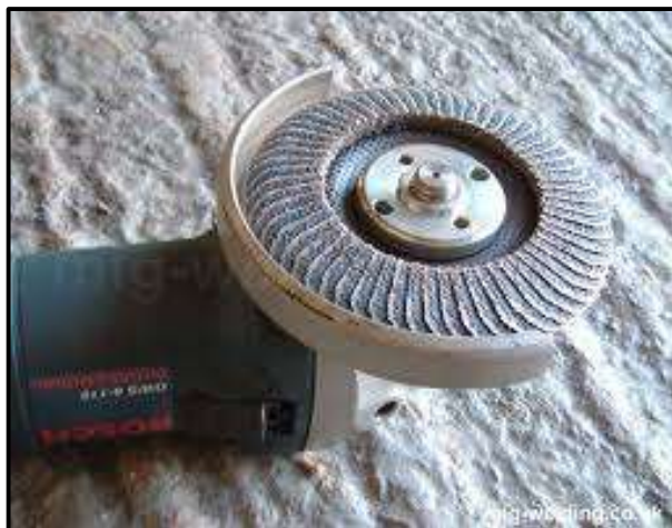
Figure 8: Flapper disc mounted on angle grinder
