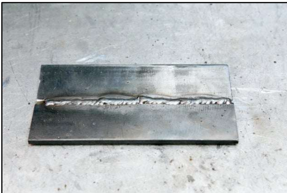
Figure 17. Completed weld runs
