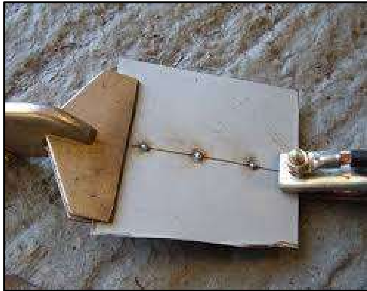
FIGURE 2: Tag weld practice piece
