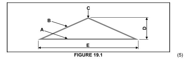
19.4 The span of a simple roof truss is 10 m and the rise is 2 m. Calculate the truss rafter. (5)
