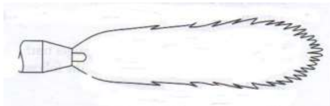
Neutral flame (Oxygen and acetylene are the same)
